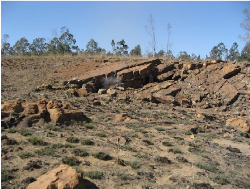
Figure 4. A collapsed, burning coal mine
